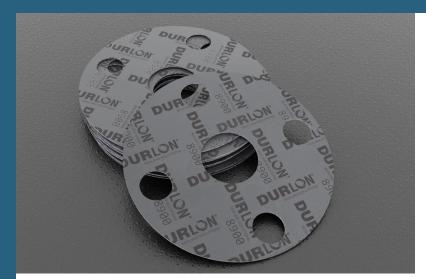
A premium grade material for service conditions to 496°C (925°F) and continuous operating temperatures of -40°C to 400°C (-40°F to 752°F). Durlon<sup>®</sup> 8900 is ideal for saturated and superheated steam, oil, dilute acids and alkalis, hydrocarbons and solvents.
