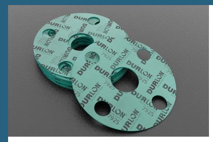
Durlon<sup>®</sup> 7925 is are an economy grade general service gasket sheet material made with NBR (Nitrile Butadiene Rubber) binder for mild service in piping and equipment with applications in steam, hydrocarbons and refrigerants and an alternative when temperature and pressure conditions are below 500°F (260°C) and 1,200 psig (See PxT chart below for validation).
