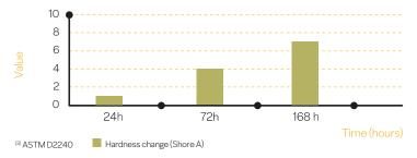
**TS 5500** low loading cork rubber material used for natural Gas and LPG applications, with good conformability to flange distortion
