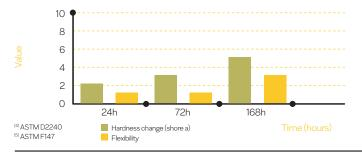
**TS 1400** sealing material is compounded with Nitrile (NBR) rubber. This product is suitable for all engine fluids and application service temperatures.
