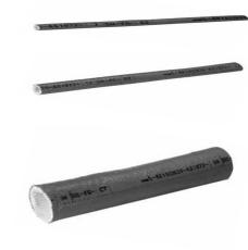
Firesleeve will protect hose from direct flame. Firesleeve is constructed of a uniform single layer of braided fiberglass tubing impregnated with flame resistant silicone rubber. Temperature range of -65°F to +500°F.
