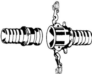
**Service:** Low and medium pressure water, petroleum and chemical transfer where fast connections are needed; also used for suction service
