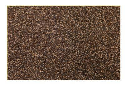
DK153/DK154 is a cork loaded sponged rubber material. DK153/DK154 is used as a gasket and dampening material in many industrial applications. Available with or without acrylic pressure sensitive adhesive. With PSA the product designation is DK153, without PSA the designation is DK154.
