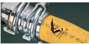
This 2" 1000 psi rated hose exploded in a test at 5200 psi. The hose exceeded its minimum 4X safety factor. The fitting and clamp exceeded the capacity of the hose.
